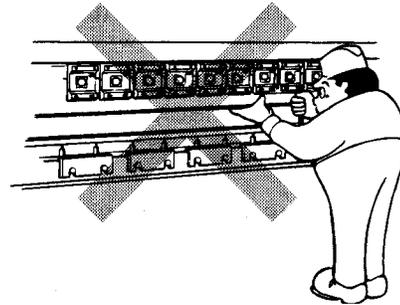
Securely fix the punches, dies, and die holders before applying any pressure to them.
