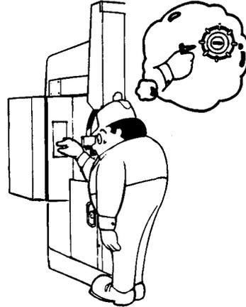
Before installing and uninstalling the punches and dies, turn the HANDWHEEL to adjust the moving beam to the desired position, turn the tool change switch to TOOL CHANGE then remove and keep the key in your possession. Never put your hands between the punches and dies to support the punches. (Install and uninstall the punches and dies as instructed in machine's operator manual.)
