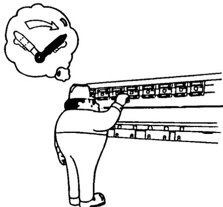
When you install and uninstall the punches and dies with an assistant operator or operators, be sure to closely coordinate and communicate with them to ensure no one is in a hazardous position.
